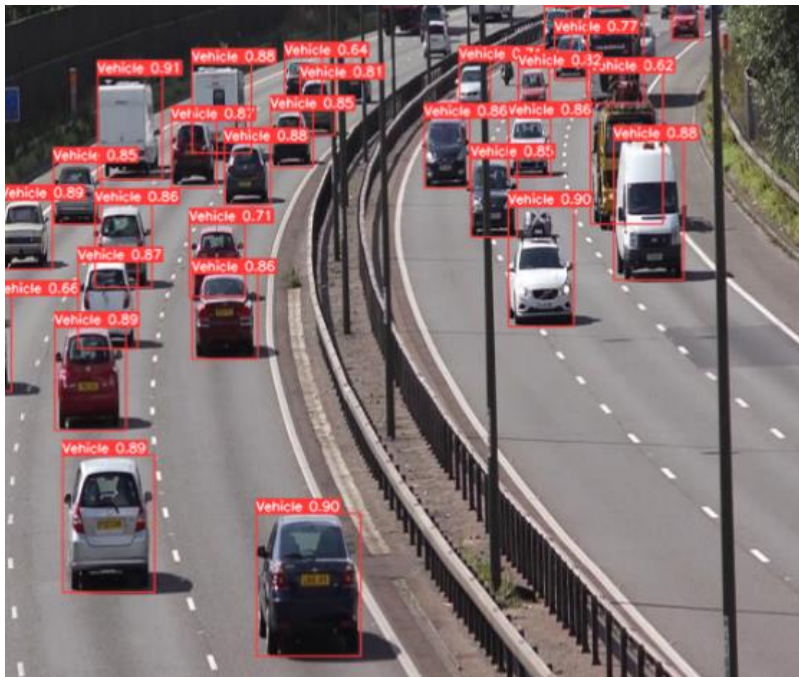
Figure 4: Vehicle detection probability-based prediction
