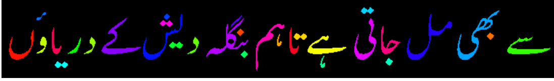
Figure 7: Segmentation of text line using connected component labelling
