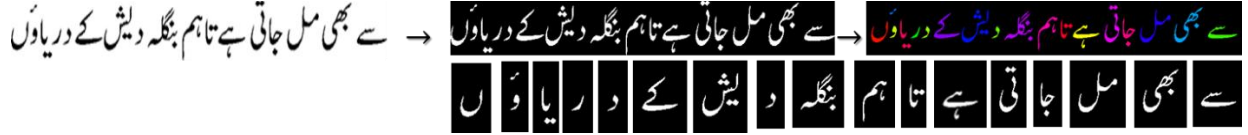
Figure 10: UPTI text line segmentation using Connected component labelling
