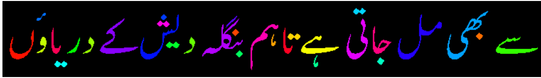
Figure 7: Segmentation of text line using connected component labelling
